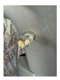
Remove front outboard seat mounts. You'll need to pull the carpet back to access one of the front seat mount bolts and depending on your truck model you'll need to keep the carpet pulled back to install the forward upright.
