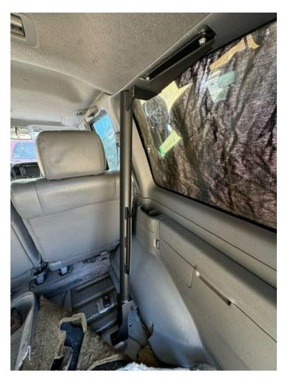
Set the forward upright in place as shown and install the top M6 bolts and small spacers first. Next, slide the lower mount into place till the lower bolt hole lines up and install the lower factory bolt. For vertical grab handles (shown) you must have the carpet pulled back and install the top bolts first. Leave all hardware loose enough for adjustment, you may need it later in the install.
