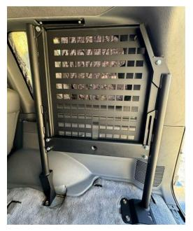
Install the cross section using the remaining M8 hardware and set to your measured height. This is where the adjustment comes in, you may need to adjust the uprights in or out till the cross section bolts line up and it moves freely up and down. Once the cross section is in and adjusted you may now fully tighten all hardware.
