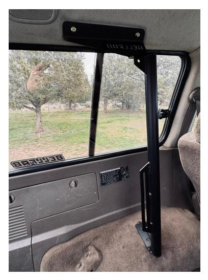
Set the forward upright in place as shown and install the top M6 bolts first. Next, slide the lower mount into place till the bolt holes line up and install the two lower M8 bolts. Depending on your carpet and padding thickness you may need to use a little force to move the lower mount in place. Thread the upper and lower bolts down but leave them loose enough for adjustment, you may need it later in the install.
