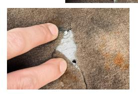
Next, set upright into place and install the two lower M6 bolts. Now install the 7/16" bolt and washer into the 3rd row seat belt hole, again you may have to push down a bit depending on carpet thickness to line up the bolt hole. Also, leave these somewhat loose allowing for minor adjustment later.
