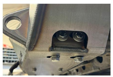
Now you can hold the wing up to the center section and install the lower 12mm bolts and then the side 10mm bolts with the larger fender washers. Leave all hardware loosely installed till the end when all pieces are installed. Repeat wing install on the other side.
