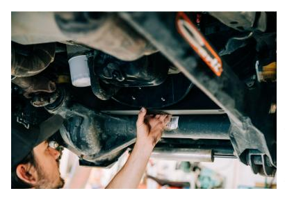
As an assembly install the front mount onto the engine crossmember by sliding the bolts through the factory holes. Install washers and nuts and snug up but do not fully tighten, you will come back at the end and fully tighten everything once it is totally assembled- This allows the skid plate to align itself.
